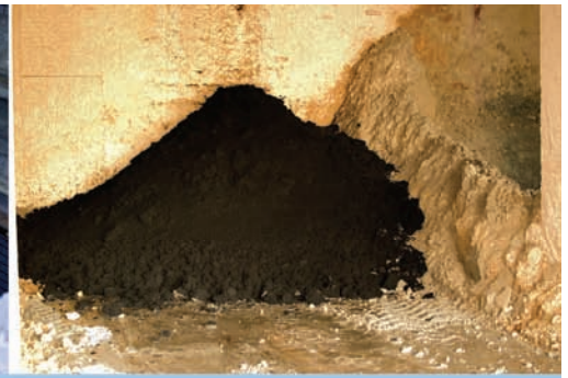
3. Finished product—dewatered sludge ready to be hauled to the landfill.
